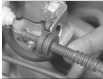
3.5b . . . then release from its support bracket
