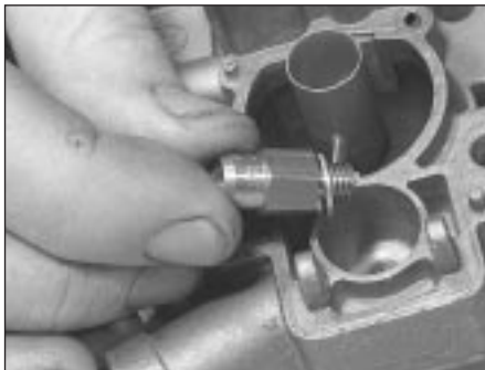
20.6c Remove the needle valve housing and its washer
