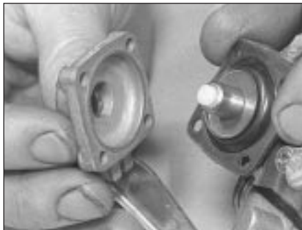
24.11a Remove the accelerator pump cover ...
