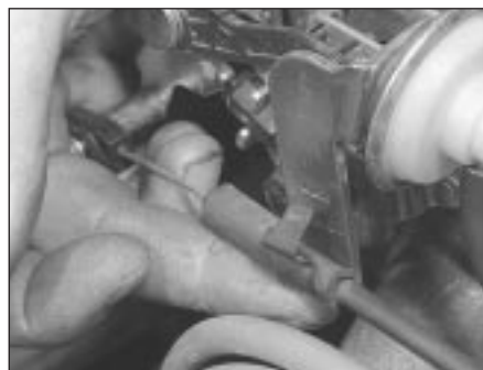
6.5b Choke outer cable retaining clip released
