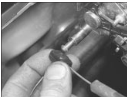
6.5a Disconnect the inner cable from the choke linkage
