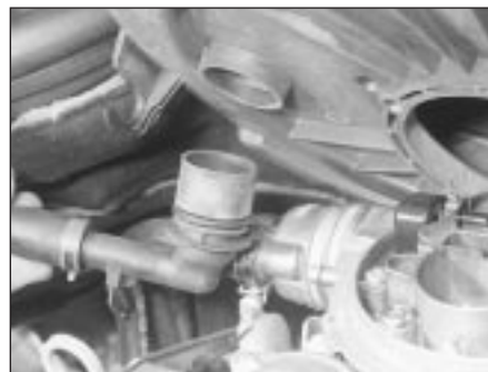
2.4a Disconnecting the oil separator/ crankcase ventilation hose from the air cleaner (CVH engine shown)
