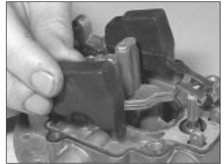
20.6b . . . then detach the float and needle valve
